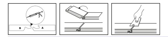
Important! Make sure that after applying the adhesive there are no gaps left between the boards.
