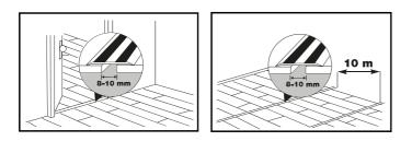
9. It is recommended that floorboards are installed so that light from the window shines parallel to the longitudinal joints of the floorboards. In this case the joints between floorboards will be less noticeable.
